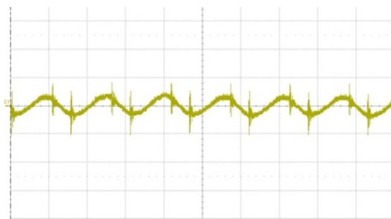
Fig. 16: Input reflected ripple current, i_s (20 mA/div.), measured through 10 \mu\text{H} at the source at full rated load current and V_{in} = 48 \text{ V} . Refer to Fig. 14 for test setup. Time scale: 2 \mu\text{s}/\text{div} .
