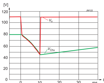
Fig. 4 Increased interruption time. V_i = 110\ V , C_{hu} = 560\ \mu F/100\ V , P_o = 90\ W , V_{oB\ tr} = 80\ V , R_{BA} = 0\ \Omega . (24IBX15-50-0G)
