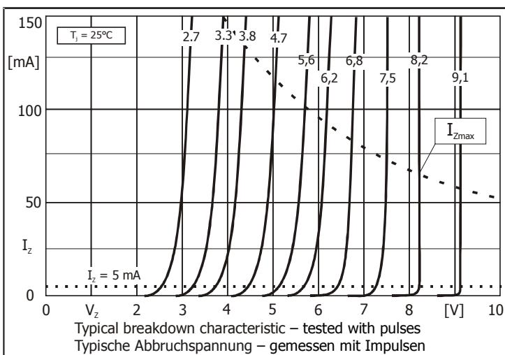
Typical breakdown characteristic – tested with pulses
