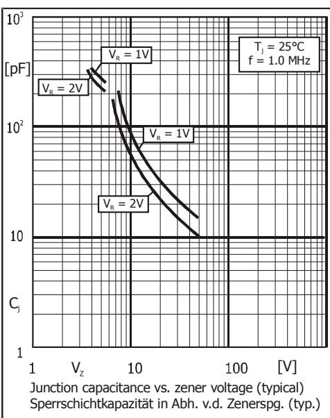
Junction capacitance vs. zener voltage (typical)
