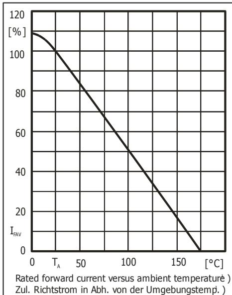
Rated forward current versus ambient temperature
