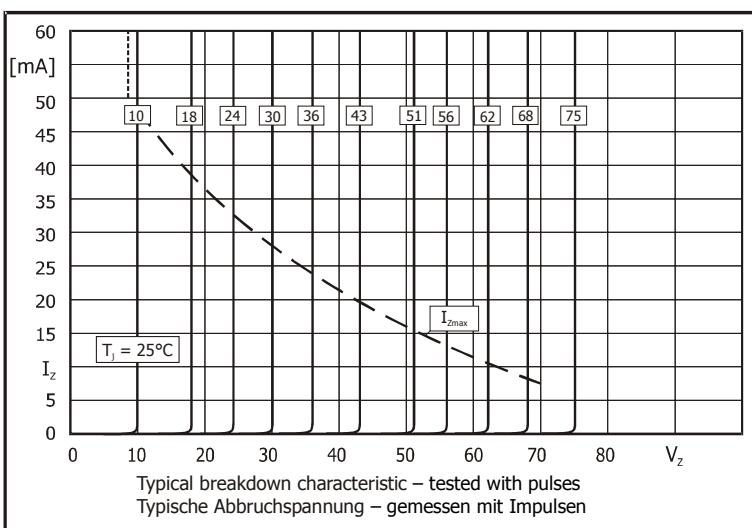
Typical breakdown characteristic – tested with pulses
