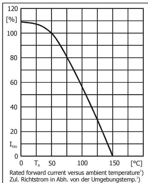
Rated forward current versus ambient temperature<sup>1)</sup>
