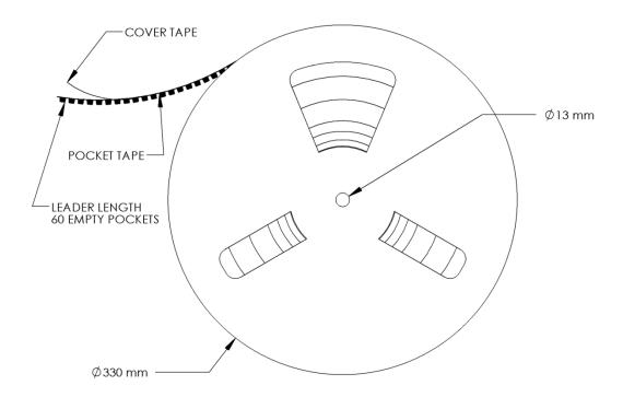
Figure 12: Emitter Reel specifications (mm).
