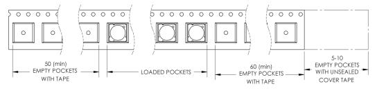
Figure 12: Emitter carrier tape specifications (mm).
