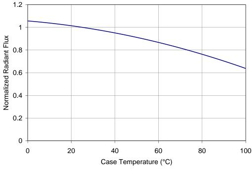
Figure 7: Typical normalized radiant flux vs. case temperature.
