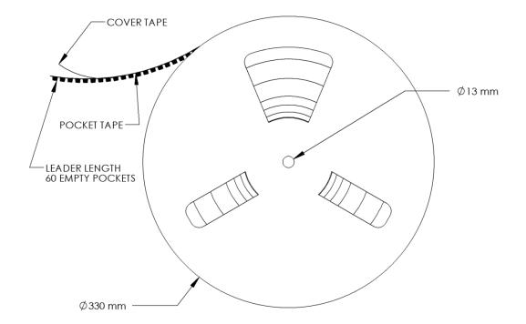
Figure 13: Emitter Reel specifications (mm).
