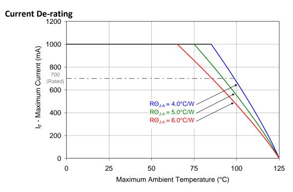
Figure 11: Maximum forward current vs. ambient temperature based on T<sub>J(MAX)</sub> = 125°C.
