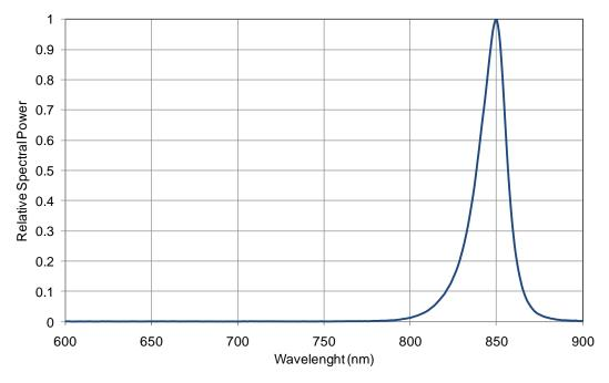
Figure 5: Relative spectral power vs. wavelength @  $T_C = 25^{\circ}C$ .
