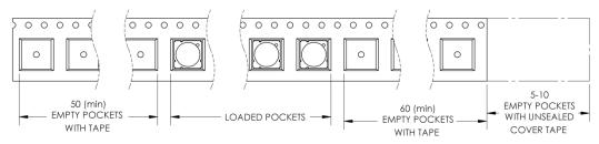
Figure 11: Emitter carrier tape specifications (mm).
