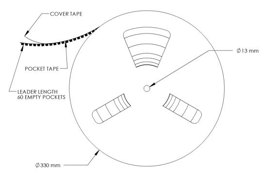
Figure 12: Emitter Reel specifications (mm).
