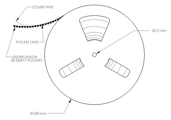
Figure 13: Emitter reel specifications (mm).
