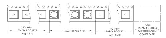
Figure 12: Emitter carrier tape specifications (mm).
