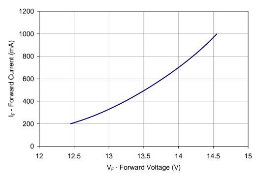
Figure 9: Typical forward current vs. forward voltage @  $T_C = 25$ °C.
