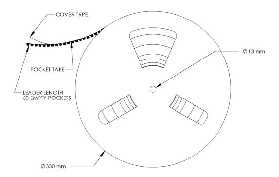
Figure 12: Emitter Reel specifications (mm).
