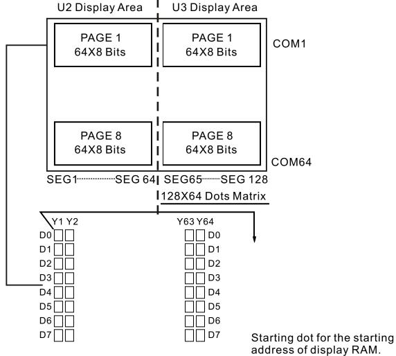
Each segment driver has 8 pages RAM, and each page has 64x8 bits RAM. D0~D7 are 8 bits transmitted data, where D0 is LSB and D7 is MSB.
