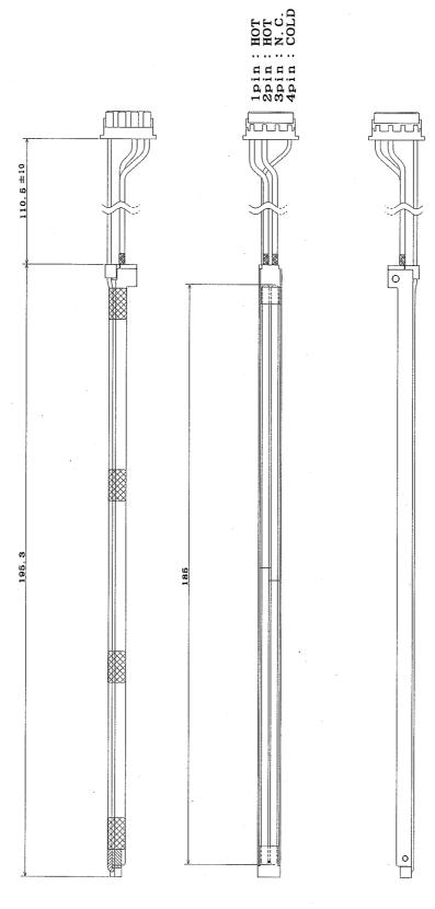
Note1: The structure of up side and down side lamp holder is the same.
