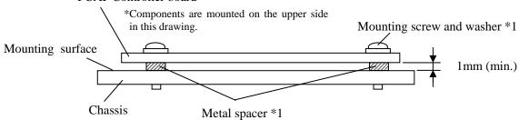
\*1: The conductive material (mounting screw, washer, metal spacer and so on) is allowed to mount within the limits of 2.5mm radius from the center of mounting hole.
