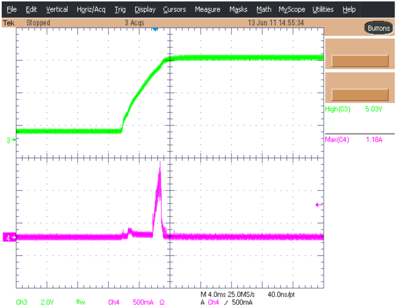
Figure 10. 12V with 5V standby power supply: inrush current at 5V
