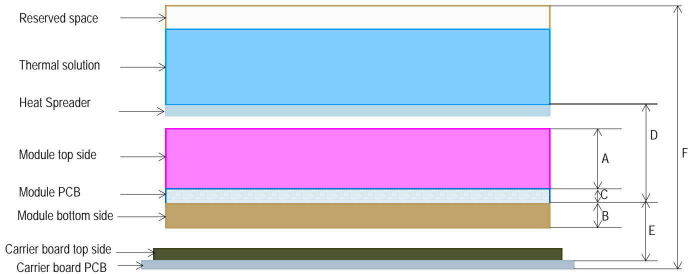
Figure 7. Height constraints of a typical system
