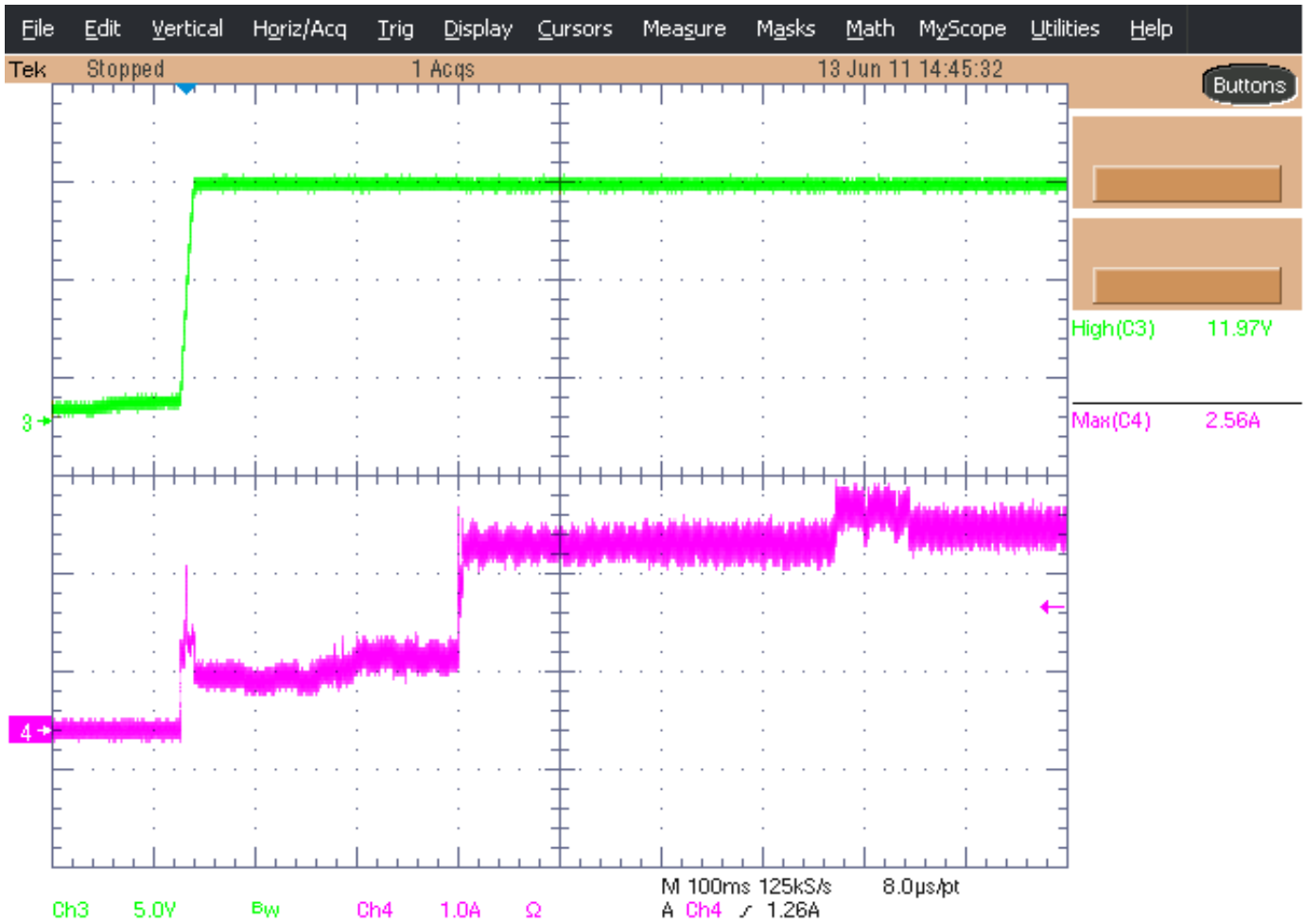
Figure 9. 12V with 5V standby power supply: inrush current at 12V
