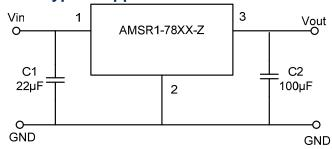
$\ensuremath{\mathsf{C1:A}}$  A low ESR capacitor is required to keep the converter to a minimum.
