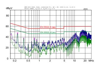
Fig. 22b Conducted emissions (peak/quasipeak and average) at the phase input according to EN 55011/22, measured at  $V_{\rm inom}$  and  $I_{\rm onom}$  (DK1601-9ERB1). The neutral line performs quite similar.
