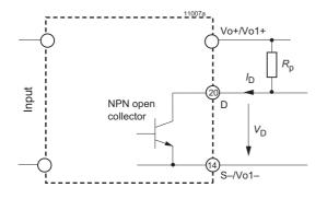
Fig. 37 Option D5 – DD: NPN output,  $V_0 \le 40$ ,  $I_D \le 2.5$  mA
