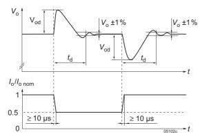
Fig. 10 Typical dynamic load regulation of  $V_0$ .
