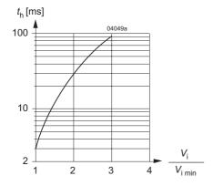
Fig. 6b Typical hold-up time  $t_{\rm h}$  versus relative AC input voltage (LK models)
