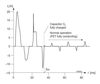
Fig. 32 Inrush current for LK models with option E (AC supply)  $V_i = 230 \text{ VAC}$ ,  $f_i = 50 \text{ Hz}$ ,  $P_0 = P_{0 \text{ nom}}$
