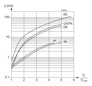
Fig. 6a Typical hold-up time  $t_{\rm h}$  versus relative DC input voltage.  $V_i/V_{i\, \rm min}$ . DC-DC converters require an external series diode in the input path, if other loads are connected to the same input supply lines.
