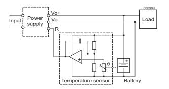
Fig. 20 Connection of a temperature sensor
