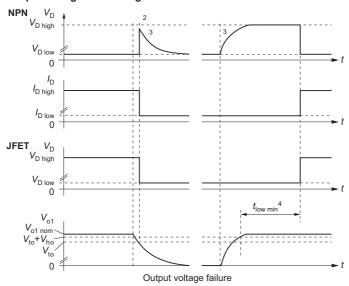
Fig. 39 Relationship between V<sub>i</sub>, V<sub>o</sub>, V<sub>D</sub>, V<sub>o</sub>/V<sub>o nom</sub> versus time
