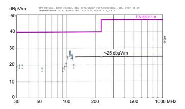
Fig. 23a Typical radiated emissions according to EN 55011/22, antenna 10 m distance, measured at  $V_{\rm i\ nom}$  and  $I_{\rm o\ nom}$  (BK1601-9R)
