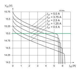
Fig. 12 Models with 2 outputs 15 V:  $V_{02}$  versus  $I_{02}$  with various  $I_{01}$  (typ)
