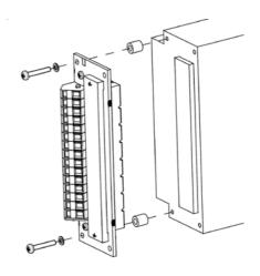
Fig. 46 Cage clamp adapter HZZ00144-G
