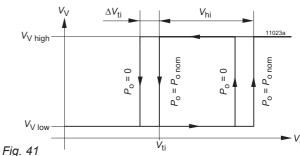
Fig. 41 Definition of  $V_{ti}$ ,  $\Delta V_{ti}$  and  $V_{hi}$
