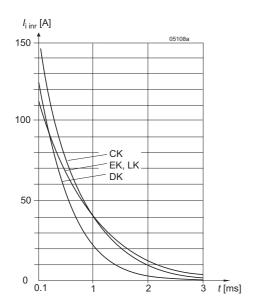
Fig. 3 Typical inrush current versus time at  $V_{i max}$ ,  $R_{ext} = 0 \Omega$ . For AK, BK, FK, and for application-related values, use the formula in this section to get realistic results.
