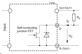
Fig. 36 Option D0 – D4: JFET output,  $I_D \le 2.5 \text{ mA}$
