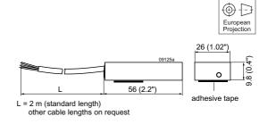
Fig. 49 Battery temperature sensor
