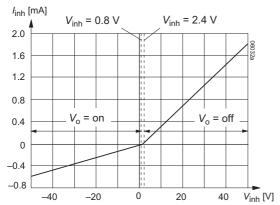
Fig. 15 Typical inhibit current I<sub>inh</sub> versus inhibit voltage V<sub>inh</sub>
