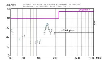
Fig. 23b Typical radiated emissions according to EN 55011/22, antenna 10 m distance, measured at  $V_{\rm i\ nom}$  and  $I_{\rm o\ nom}$  (DK1601-9ERB1)
