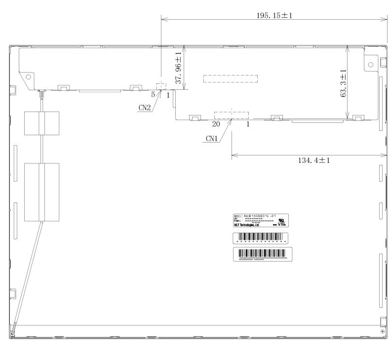
Note1: The torque for product mounting screws must never exceed 0.392N·m. And the length of product mounting screws must be  $\leq 4.5$  mm.
