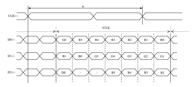
(3) LVDS Input data signal: 6bit (MSL: High, FRC: High or Open)
