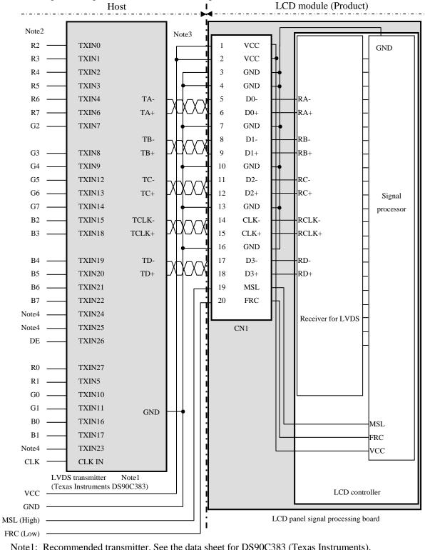
4.5.4 Connection between receiver and transmitter for LVDS
