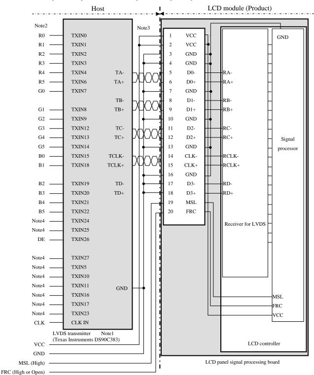
(3) LVDS Input data signal: 6bit (MSL: High, FRC: High or Open)
