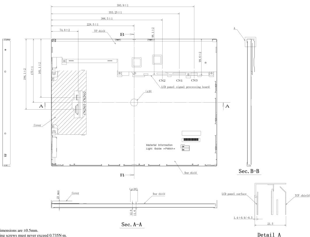
Note1: Not shown tolerances of the dimensions are  $\pm 0.5$ mm.
