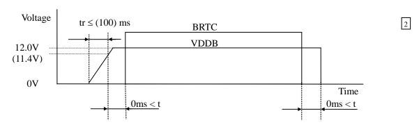
Note1: The backlight should be turned on within the valid period of LVDS signals, in order to avoid unstable data display.
