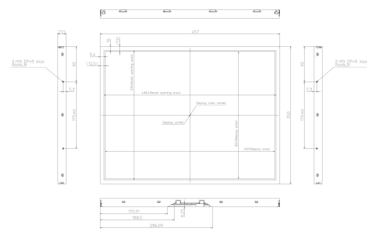
Note1: Not shown tolerances of the dimensions are  $\pm 0.5$ mm.
