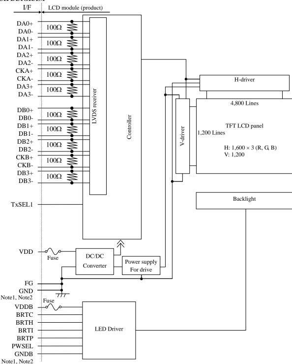
Note1: Relations between GND (Signal ground), FG (Frame ground) and GNDB (LED driver board ground) in the LCD module are as follows.
