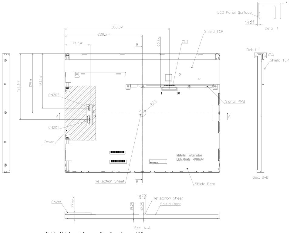
Note1: Not shown tolerances of the dimensions are  $\pm 0.5$ mm.
