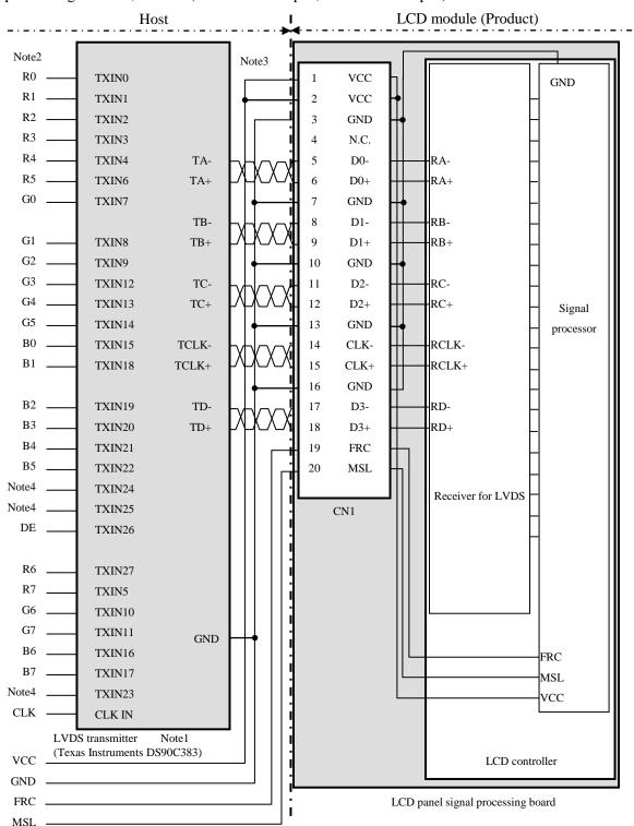
(2) Input data signal: 8-bit, MAP B (MSL: Low or Open, FRC: Low or Open)
