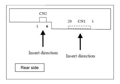
4.5.4 Connection between receiver and transmitter for LVDS
