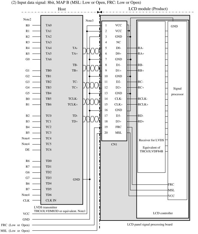
Note1: Recommended transmitter THC63LVDM83D (THine Electronics Inc.) or equivalent
