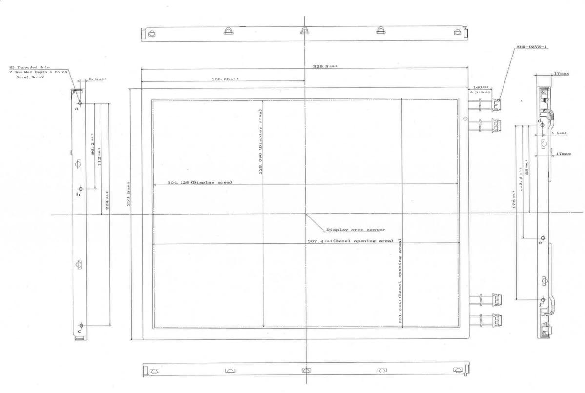
Note1: The torque for product mounting screws must never exceed 0.343 N·m. And the length of product mounting screws must be  $\leq$  2.8mm. Note2: NEC's reliability tests are carried out using mounting holes "a", "c", "d" and "f".
