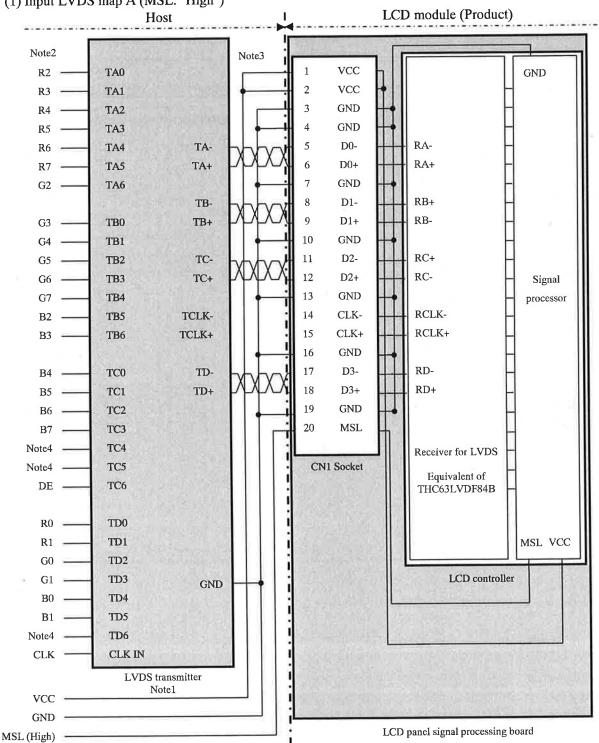
4.5.4 Connection between receiver and transmitter for LVDS (1) Input LVDS map A (MSL: "High")
