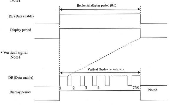
Note1: This diagram indicates virtual signal for set up to timing. Note2: See "**4.9.3 Input signal timing chart**" for numeration of pulse.
