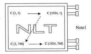
Note1: Meaning of C (X, Y) C (X, Y): The coordinates of the display position (See "4.7 DISPLAY POSITIONS".)
