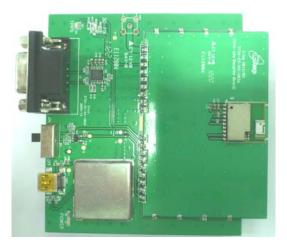
Built-in chip antenna (series 4): Gms-g6、Gms-b6(Common board)
